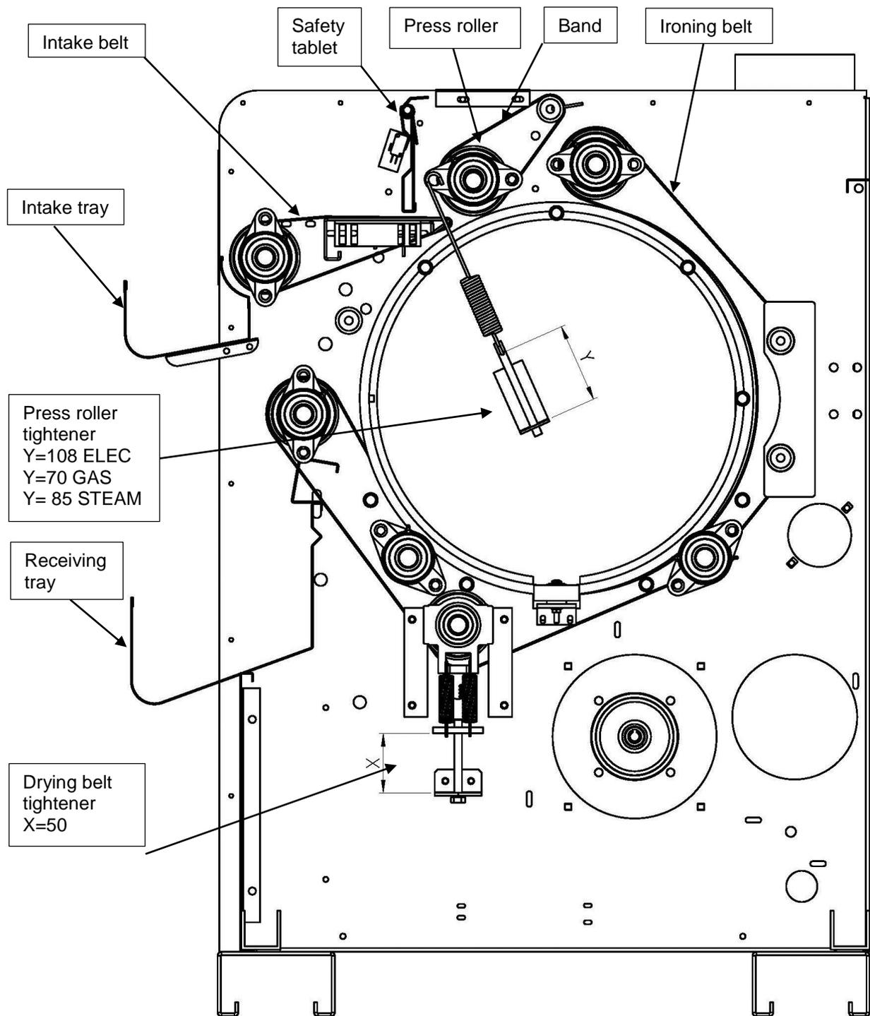
When the laundry is placed flat on the table at the front of the machine, it is automatically taken to the drying and ironing cylinder by means of the nomex-polyester belts.
