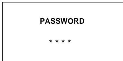
To access the user menu you must enter code 1-3-5-7. Use keys INC (^) and DEC (v) to change the digits and with the SELECT key you can go from one digit to another. When the four figures have been entered, press SELECT to go to the User menu.
