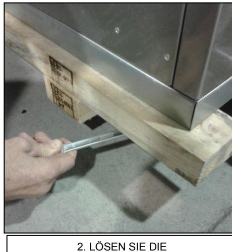
2. LÖSEN SIE DIE SCHRAUBENSchlÜSSEL No. 17
