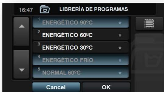
Use the “up arrow” and “down arrow” keys to change the position of any programme in the list of favourites, which can be arranged in any order required.
