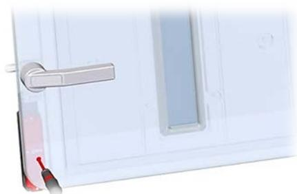
Access the door safety device through the hole provided at the bottom left of the porthole, **then unlock.**
