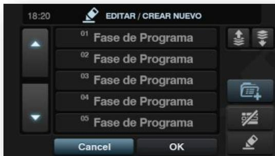
Cycles can be added in the cycles library. The cycles you wish to view can be filtered by cycle type. After you have selected the cycle, the cycle library parameters can be consulted before including them in the programme you are creating.
